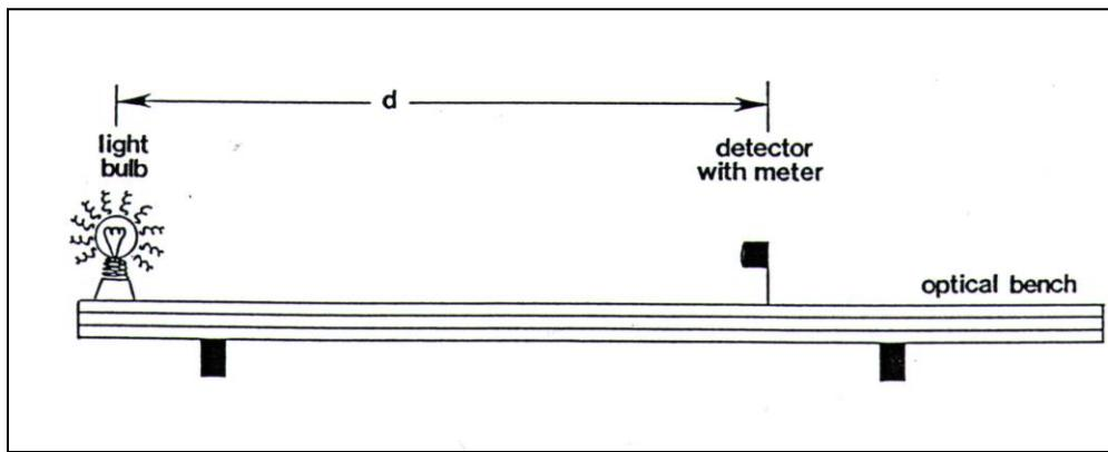
Figure 2. Laboratory setup for measuring intensities in inverse-square law experiment.
